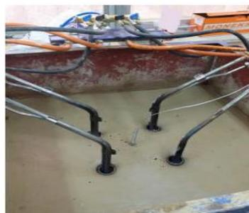
**Figure 2.** Soil improvement using Heaters (Rahil, 2019)
