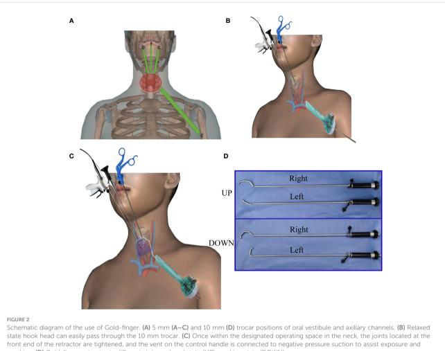
smoking. (D) Gold-finger retractor in different states; relaxed state (UP), working state (DOWN).
