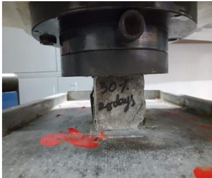
Figure 2: Compressive Strength Test
