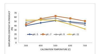
Figure 3. Impurities content in product with calcium carbonate rock material
