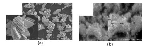
Figure 4. SEM Image of precipitated CaO prepared by blood clam shells at (a) pH 7 and (b) pH 11
