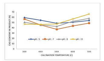
**Figure 2.** The effect of pH and the temperature of calcination on the CaO content in the precipitated CaO prepared by limestone
