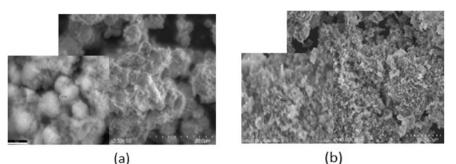
Figure 5. SEM Image of precipitated CaO prepared by carbonate rock material at (a) pH 7 and (b) pH 11
