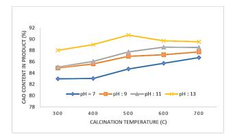
**Figure 1.** The effect of pH and the temperature of calcination on the CaO content in the precipitated CaO prepared by clam blood shells
