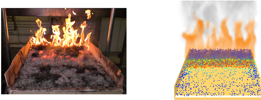
Fig. 2. Example of (left) experiment and (right) simulation, with particles colored by temperature and fire represented by local heat release rate and soot concentration. This is intended for qualitative illustration only, in order to present the physical scenario under consideration.
