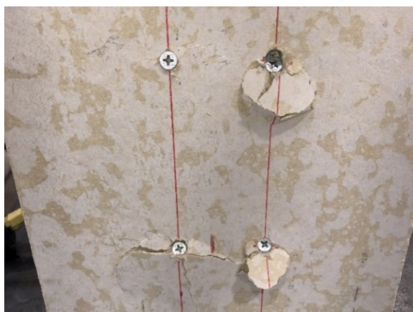
Figure 11 Unsymmetrical failure for a back-to-back specimen
