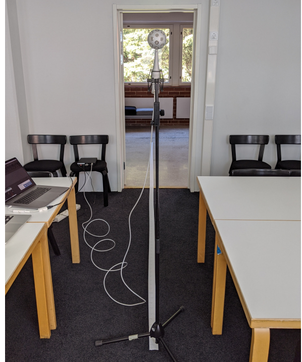
Fig. 2: Impulse response measurement setup for the Meeting Room to Hallway transition with a spherical microphone array and a loudspeaker. The tape on the floor indicates the microphone positions.
