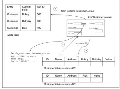
Figure 1. Multi-Schema Concept
