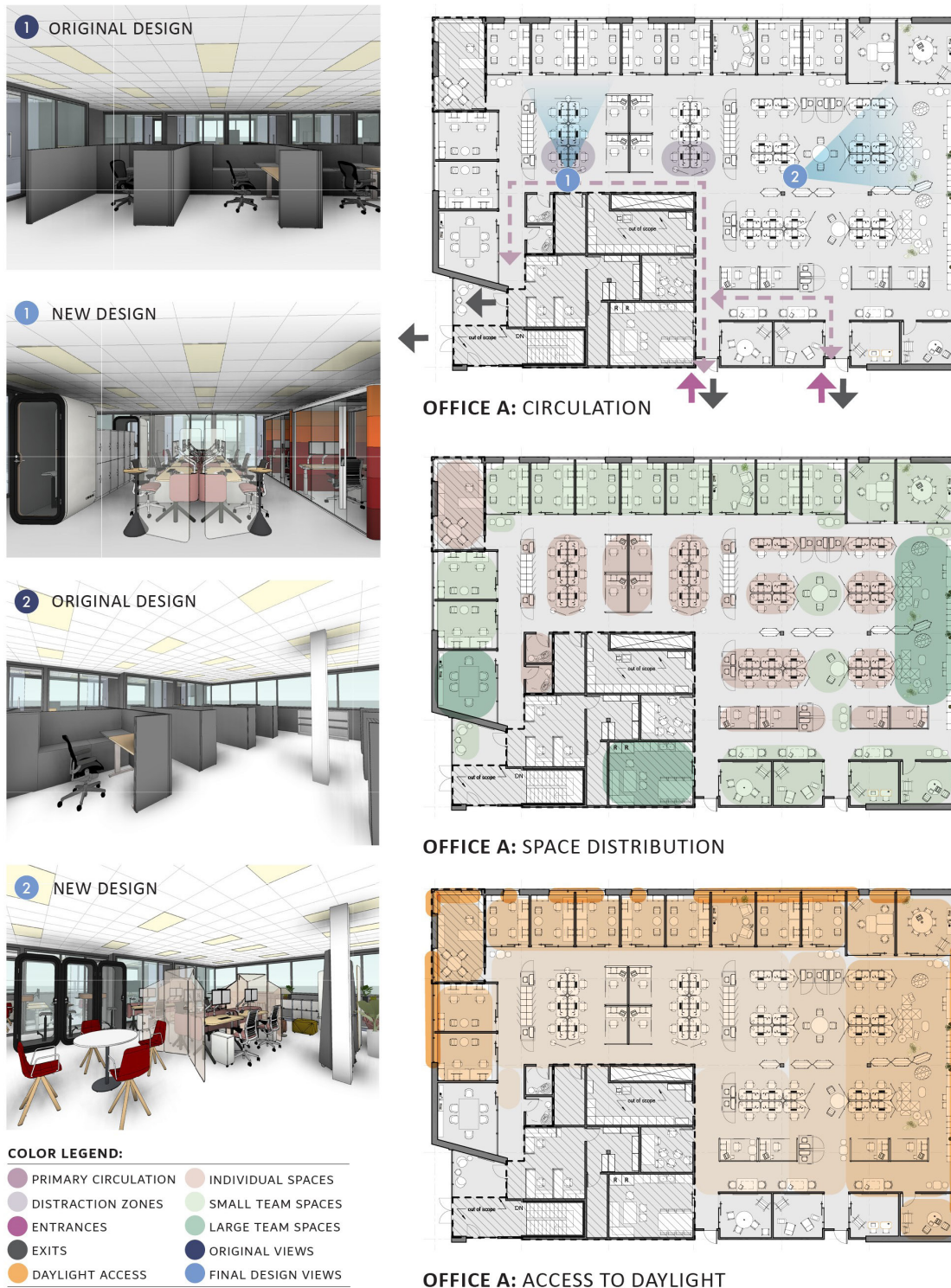
Figure 13: Office A final design plan diagrams and interior views that illustrate original and new design strategies.
