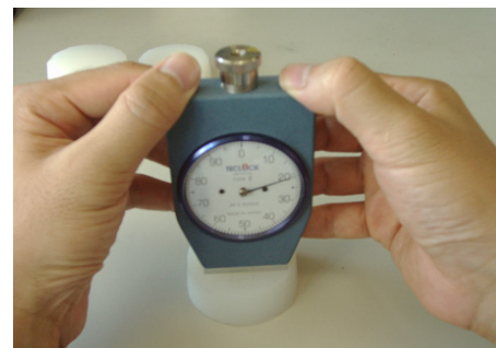
Figure 8. Measurement of silicon specimens by using a durometer scale
