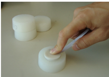
Figure 7. Measurement of silicon specimens by using MSS
