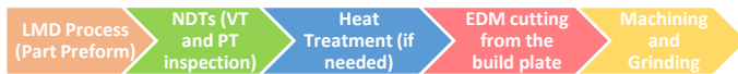
FIGURE 8: New manufacturing route by laser metal deposition with the NiCrSiFeB alloy C proposed.
