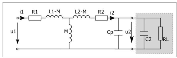
Fig 2 ECD of Magnetic Coupled RFID Reader Coil and Transponder Coil
