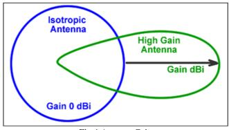
Fig 4 Antenna Gain
