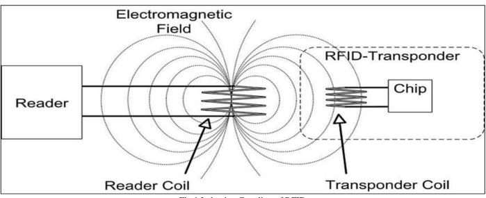
Fig 1 Inductive Coupling of RFID
