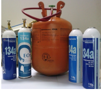
Figura 23: Gases refrigerantes, tetrafluoretano 134 a e pentafluoretano 404a.
