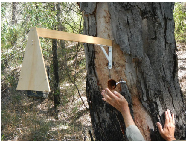
Figure 1. Camera mounted on a bracket attached above a drilled hole giving access to internal void allowing the camera to photograph inside the entrance and adjacent area of the trunk. String to the side is attached to a temperature logger.
