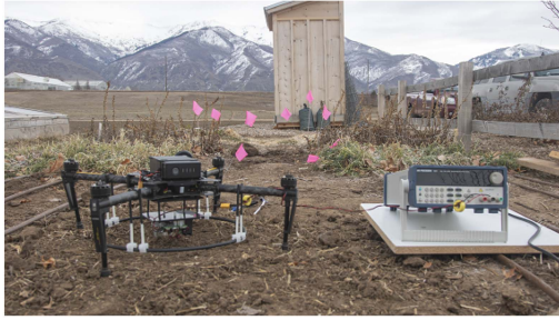
Fig. 23. Photograph of an M100 drone performing HF-IPT through the soil in a trial in an agricultural field.
