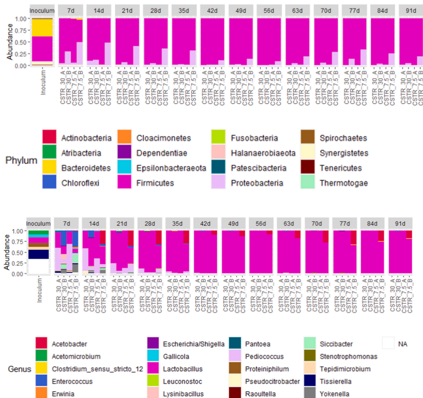
Fig. 8. Evolution of the microbial community in CSTR runs 30 A, 30 B, 7.5 A, 7.5 B. Abundance of top 16 taxa at phylum level and top 20 taxa at genus level at each timepoint (days 7 – 91) and in each CSTR.
