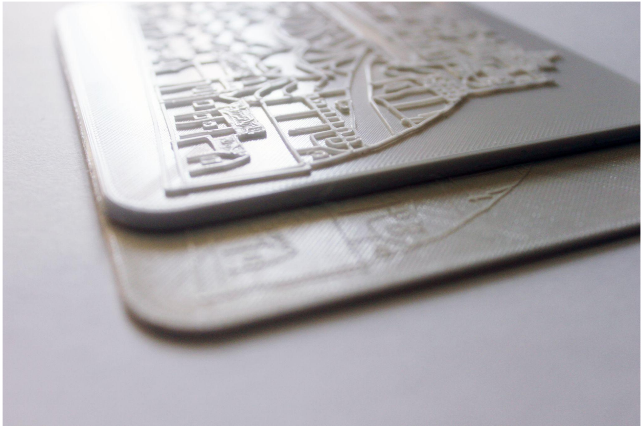
Fig. The image above pictures two versions of the same 3D printed tactile image of the oldest image of Venice. The thicker plate is placed on top of the other and is photographed from the side at an extreme angle, showcasing a substantial difference in plate bed thickness with the print on the bottom being 0.5mm in thickness and the other print being 1.5mm.
