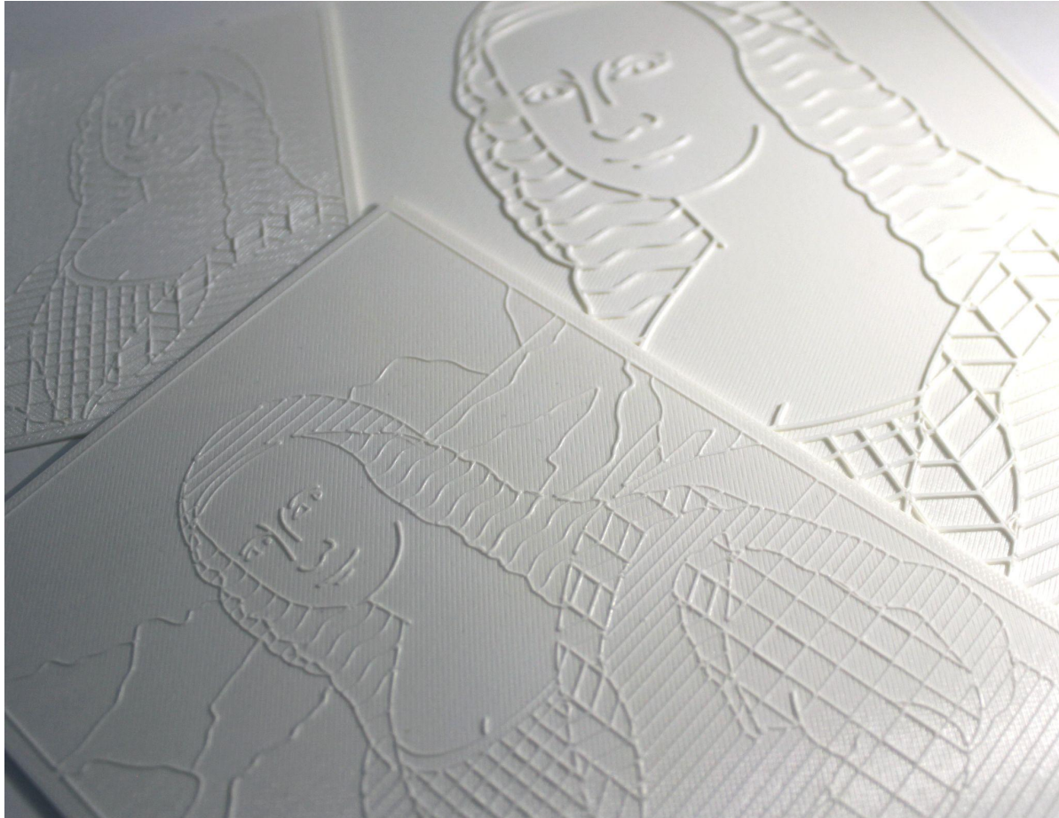
Fig. 22: The image above pictures three tactile renditions of the Mona Lisa, all three of which are printed in white PLA plastic. These two and half dimensional images are constructed with the texture swatches referenced in earlier chapters, with a wave pattern denoting the texture of the hair and a variety of line and grid patterns denoting fabric.
