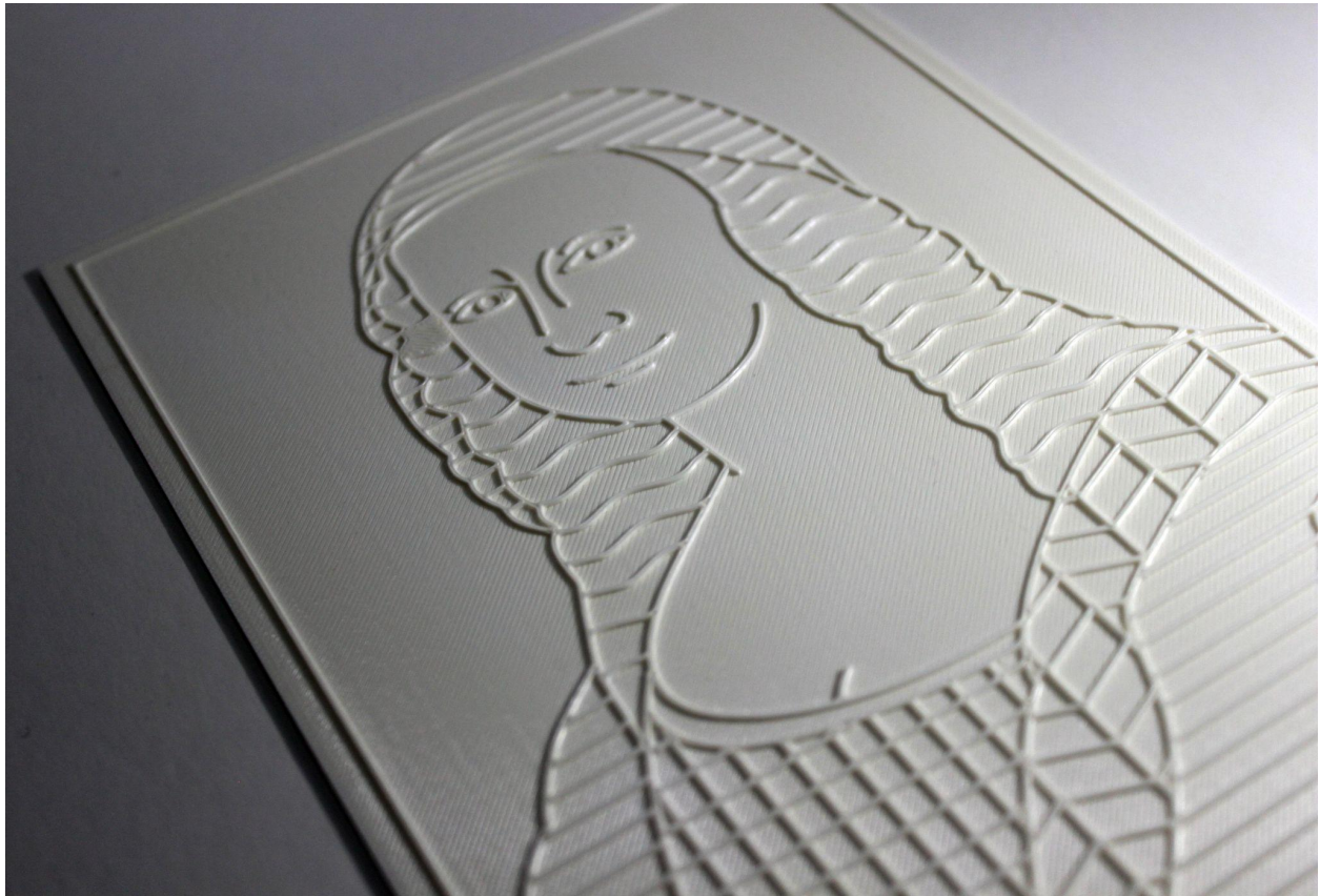
Fig. 23: The accompanying image pictures a tactile version of the Mona Lisa, printed with a raised line height of 0.5mm. All background detail is omitted and only a section of the figure is present, depicting the upper portion of the woman in a bust like style. A frame encases the portrait, making sure each texture is contained within its own section and minimising sharp terminator points that can come from the endpoints of 3D printed lines.
