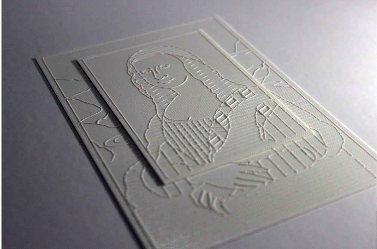
Fig. 25: The image above shows both of the tactile renditions of the Mona Lisa that feature a 0.25mm line height. The smallest cropped version is placed on top of the more complete image, in such a way that some lines connect to the image below, highlighting exactly where the image has been cropped and that the sizing between the two has remained consistent.
