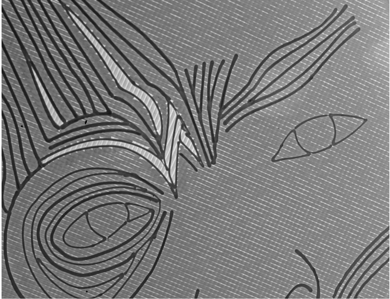
Fig. 18: Is a close up of my 'Vandeventer and Patterson' line print, backlit in such a way that the thinnest parts of the printed plate appear lighter, showing the areas where the print was close to failing. This demonstrates areas of concern, which suggest the thickness of the plate should be slightly increased on future prints.
