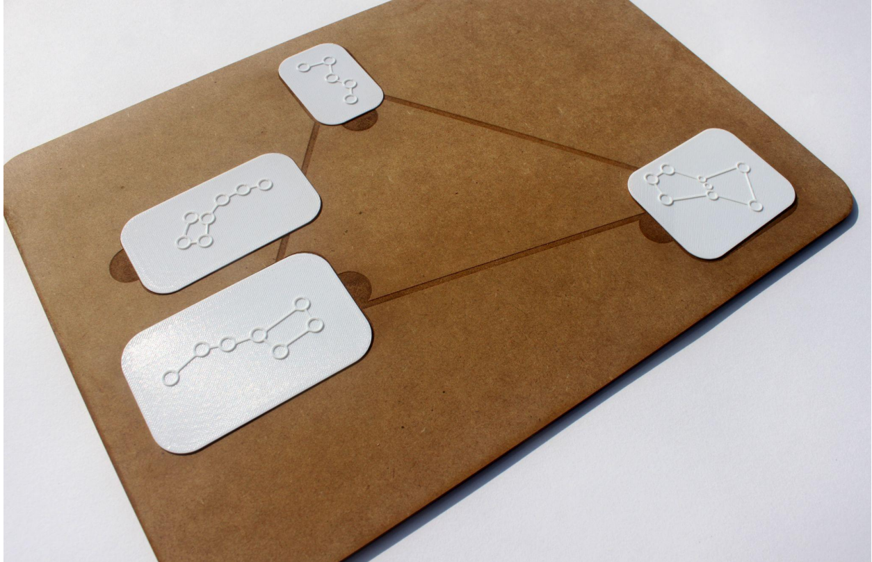
Fig. 20: The first image documents four 3D printed constellations, Cassiopeia, Orion, and both Ursa Minor and Major. Circles indicate the stars themselves with each star in a constellation being connected by the lines that make up their imagined form. The second image shows the same four prints presented on an MDF board, etched lines and rounded squares highlight where prints should be placed in order that their placement in the night sky can be understood in relation to one another. Cassiopeia is placed top centre of the board, Ursa Minor below and to the left of Cassiopeia, Ursa Major is below and slightly to the left of Ursa Minor, and Orion is located bottom right of the board, it being the constellation furthest removed from the others.
