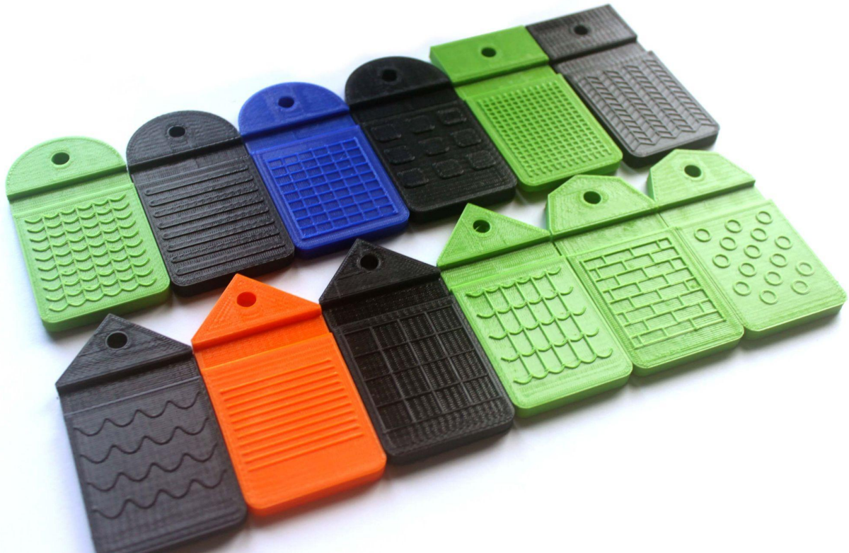
Fig. 10: Is an image of all twelve successful swatches, each model and printed by myself as their own OOR. A variety of colours of PLA and 'head shapes' are present which is reflective of the prototype nature of these test prints.
