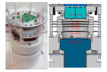
FIG. 2. Image (left) and solid model cross section (right) of the XELDA TPC. In normal operation, the liquid surface sits midway between the anode and gate grids. The liquid level is measured at three locations via the capacitance between pairs of copper plates—the bottom plate of one pair is visible in the center of the image on the left.
