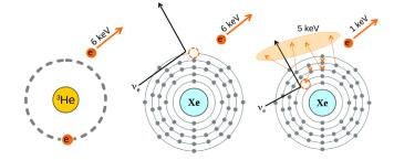
FIG. 1. A diagram depicting a  $\beta$  decay from tritium (left), a valence recoil from neutrino or Compton scattering (center), and an inner-shell recoil (right). Each of these interactions deposits a total of 6 keV via electron recoil(s), but the inner-shell recoil produces a distinct event topology from either the  $\beta$  decay or valence recoil.
