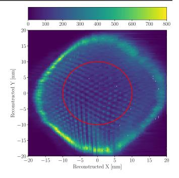
FIG. 6. Reconstruction of (x, y) position based on the S2 hit pattern in the top PMTs for *K*-shell events. The honeycomb pattern imprinted by the focusing of electrons as they drift past the gate grid is clearly visible inside the fiducial volume. The red circle indicates the radial extent of the fiducial region of the TPC (10 mm).
