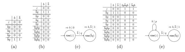
Figure 3.2: An example run of  $GL^*$  for the target language  $[(while \ b \ do \ p); q]$
