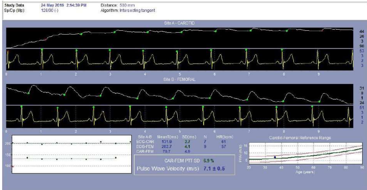
Figure 2-11: Representative output of pulse wave velocity from the SphygmoCor device.
