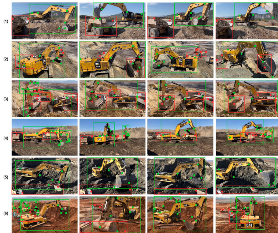
Fig. 8. The visualisation of the output of the machinery keypoint-RCNN model. Scenarios (1) and (5) contain an excavator and a dumper; Scenario (2) includes an excavator and multiple dumpers. Scenarios (3), (4) and (6) contain multiple excavators and multiple dumpers. In each example, the green rectangle describes the bounding box of excavators, and the red one describes that of dumpers. The green dots represent the keypoints of excavators, and the red dots represent the keypoints of dumpers.
