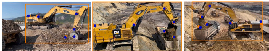
Fig. 9. The comparison of the output of the machinery keypoint-RCNN model (orange dots) and ground truth (blue dots).
