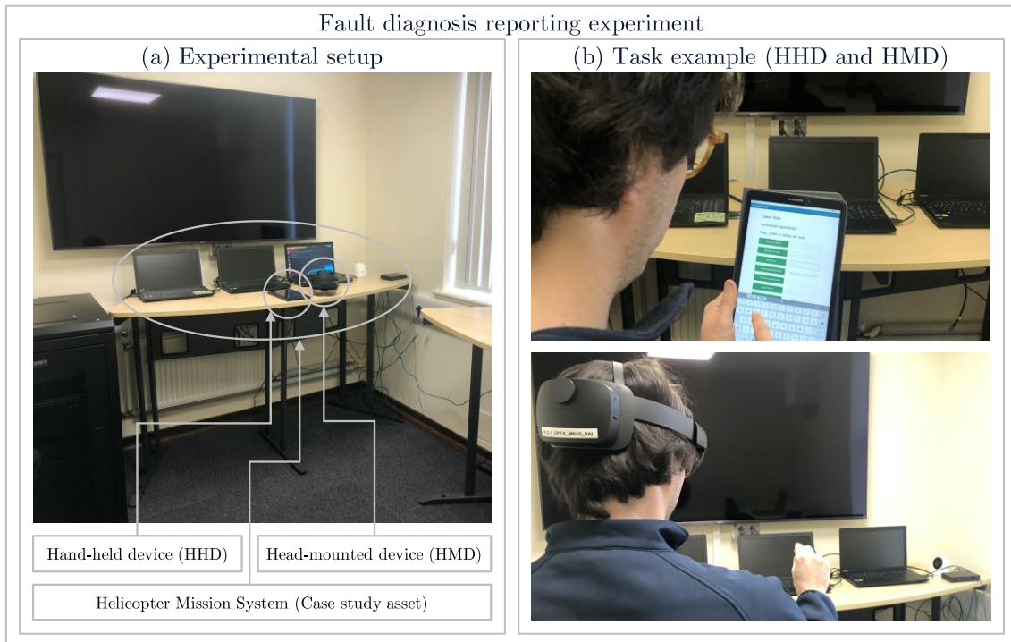
Figure 5-10. Description of diagnosis reporting experiment: (a) experimental setup and (b) task examples with hand-held (HHD) and head-mounted (HMD) devices.
