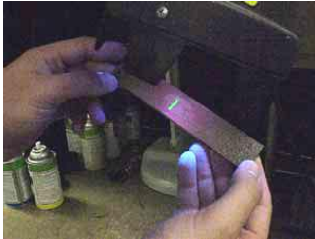
Figure 2-3 Example of testing by dye penetrant method [30]
