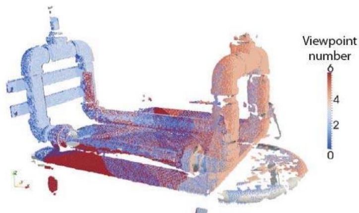
Figure 2-42 The sample of 3D images by mapping the geometry of the object with the thermal [94]
