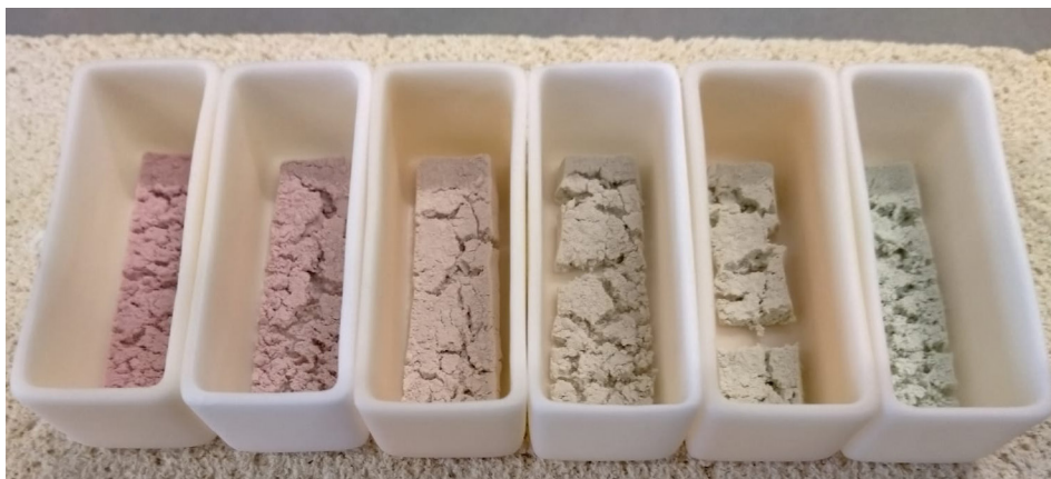
Figure S6-1. \text{NaSc}(\text{Si}_{1-x}\text{Ge}_x)_2\text{O}_6 : \text{Cr}^{3+} 1% from left to right were x=1.0, 0.8, 0.6, 0.4, 0.2, 0.0 direct after annealing
