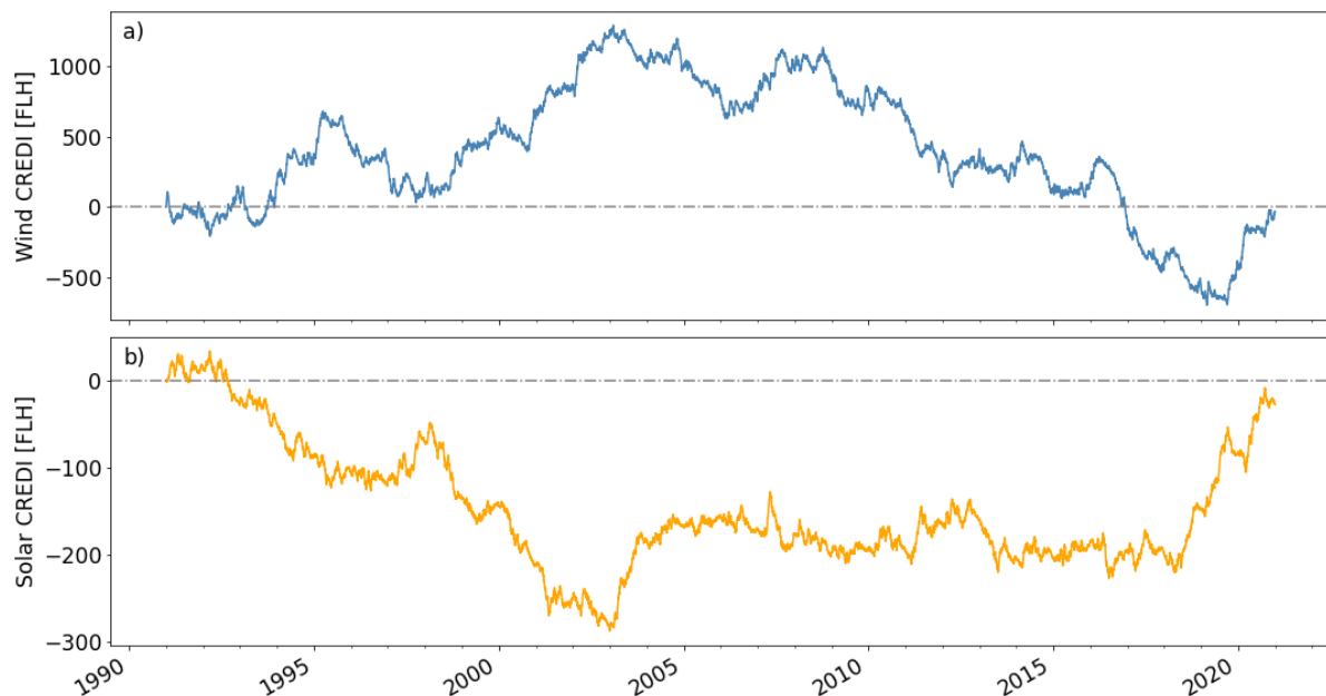
Figure S22: As Figure 4 in the main text, but then for the South-East of France ('FR10'). Hourly Wind (a) and Solar (b) CREDI over the period 1991-2020 for 'NL01'. As the climate was calculated over the same period, by definition the CREDI sums to zero over the full period.
