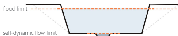
fig. 53: Flood limit can be enhanced by wider riverbed and absorbing surfaces (by author):
