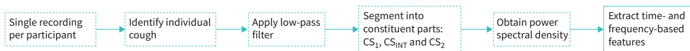
FIGURE 2 Flowchart showing the key analysis methods applied to the cough sound recordings from study participants. CS 1 : first cough sound; CS 2 : second cough sound; C INT : intermediate part of cough sound.
