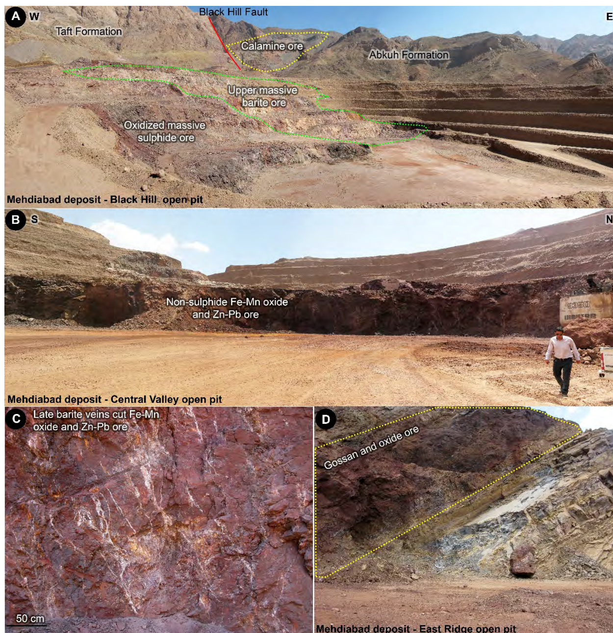
Figure 4: Outcrop views from Black Hill open pit and Calamine ore (A), Central Valley (B) and East Ridge (D) open pits in Mehdiabad giant deposit, representing oxidized massive ore, upper massive barite, non-sulphide Fe-Mn oxide and Zn-Pb ore, and late barite veins (C).
