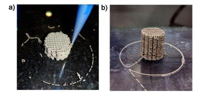
**Figure 7.** Sample production (images provided by AMES Medical): (**a**) image of the printing process to produce (**b**) porous Ti cylinders.
