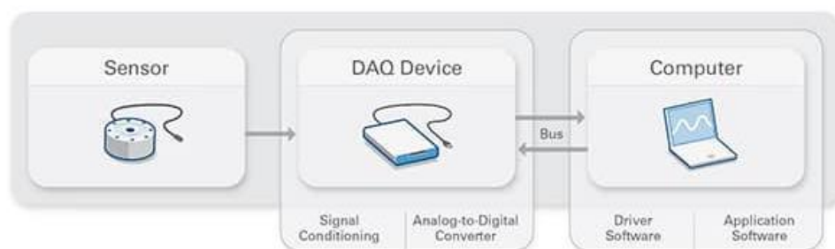
Figure 6. DAQ system scheme (Source: Internet [9])
