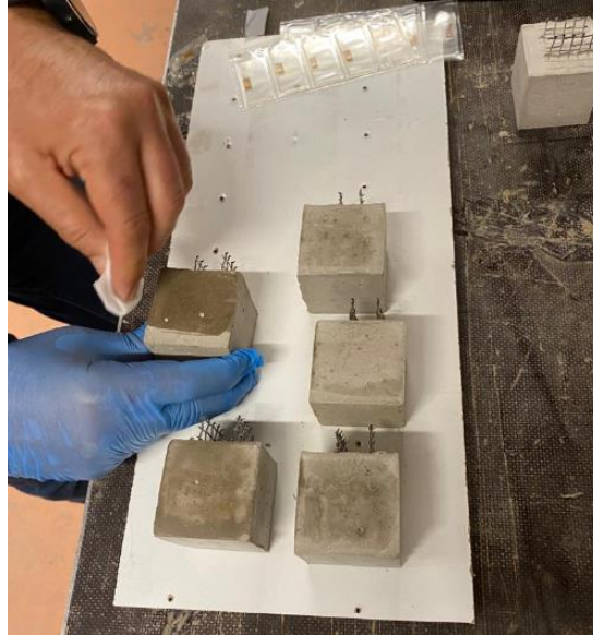
Figure 47. Cleaning of the specimens (Source: Own)
