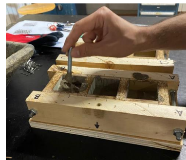
Figure 42. Compaction of the cement (Source: Own)
