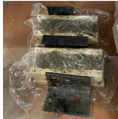
Figure 45. Specimens left to dry with a plastic cover (Source: Own)
