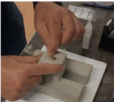
Figure 48. Installation of a gauge (Source: Own)
