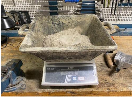
Figure 39. Cement weighing (Source: Own)
