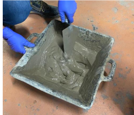
Figure 40. Cement and water mixing (Source: Own)
