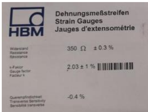
Figure 50. Gauges datasheet (Source: Fabricator)
