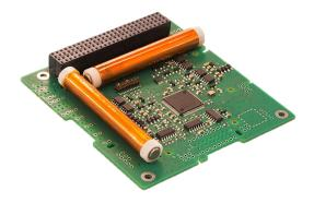
Figure 2.11 Magnetorquers implemented on a PCB. (Source: [18])
