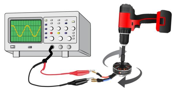
Figure 3.1 Experimental way to know the optimal waveform of a motor. (Source: own)
