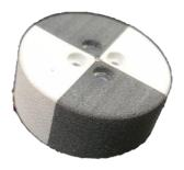
Figure 4.4 Flywheel manufactured by UPC Terrassa 3D printer. (Source: own)
