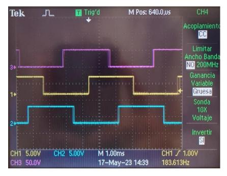
Figure 5.13 Sensor output signals obtained. (Source: own)
