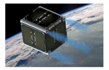
Figure 2.13 Thrusters on a CubeSat. (Source: [20])
