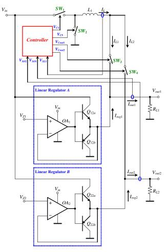
Fig. 4. Basic structure of a SIDO linear-assisted DC/DC converter.
