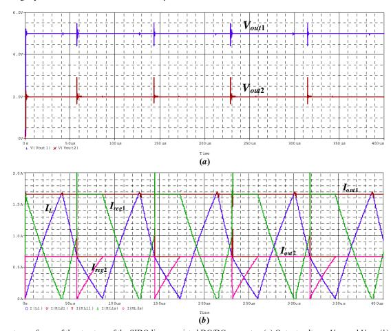
Fig. 7. Current waveforms of the structure of the SIDO linear-assisted DC/DC converter: (a) Output voltages  $V_{out1}$  and  $V_{out2}$ . (b) Currents of interest in the circuit:  $I_L$ ,  $I_{reg1}$ ,  $I_{reg2}$ ,  $I_{out1}$  and  $I_{out2}$ .
