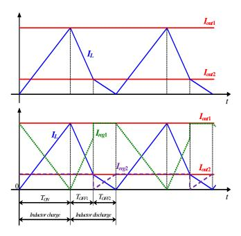
Fig. 5. Current waveforms of the SIDO linear-assisted DC/DC converter with control strategy A: through the load 1 and load 2 (red color traces), inductance  $L_1$  (blue trace), linear regulator 1 (discontinuous green trace) and linear regulator 2 (discontinuous violet trace).
