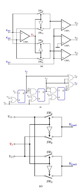
Fig. 6. Structure of the controller block for the SIDO linear-assisted DC/DC converter: (a) Generator of the internal threshold levels for the state machine. (b) State machine that generates the control signals  $V_{C1}$ ,  $V_{C5}$ ,  $V_{Cout1}$  and  $V_{Cout2}$  for the switches  $SW_1$ ,  $SW_2$ ,  $SW_3$  and  $SW_4$ , respectively. (c) Block to decide which of the two outputs (switch  $SW_3$  or  $SW_4$ ) is selected first within the inductor discharge interval.
