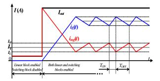
Fig. 3. Principle of operation of the proposed linear-assisted DC/DC converter.
