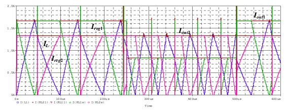
Fig. 8. Current waveforms of the structure of the SIDO linear-assisted DC/DC converter when the output current  $I_{reg1}$  changes from 1.67 A to 0.83 A at  $t=250 \mu s$  and vice versa at  $t=500 \mu s$ . Currents of interest in the circuit:  $I_L$ ,  $I_{reg1}$ ,  $I_{reg2}$ ,  $I_{out1}$  and  $I_{out2}$ .
