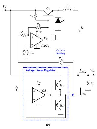
Fig. 2. (a) Block diagram of the proposed linear-assisted converter.(b) Basic structure of the proposed linear-assisted DC/DC converter.
