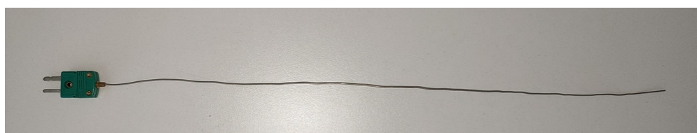
Figure 18: Thermocouple covered with inconel
