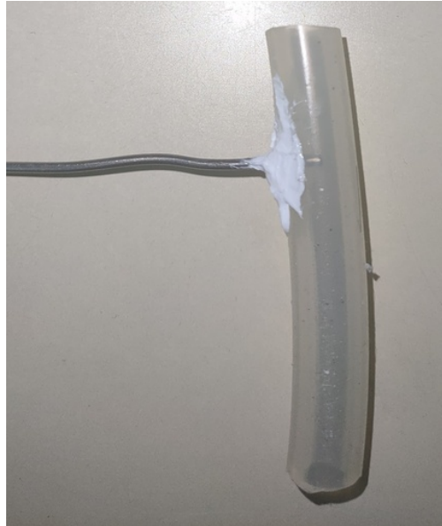
Figure 20: Thermocouple installed in pipe
