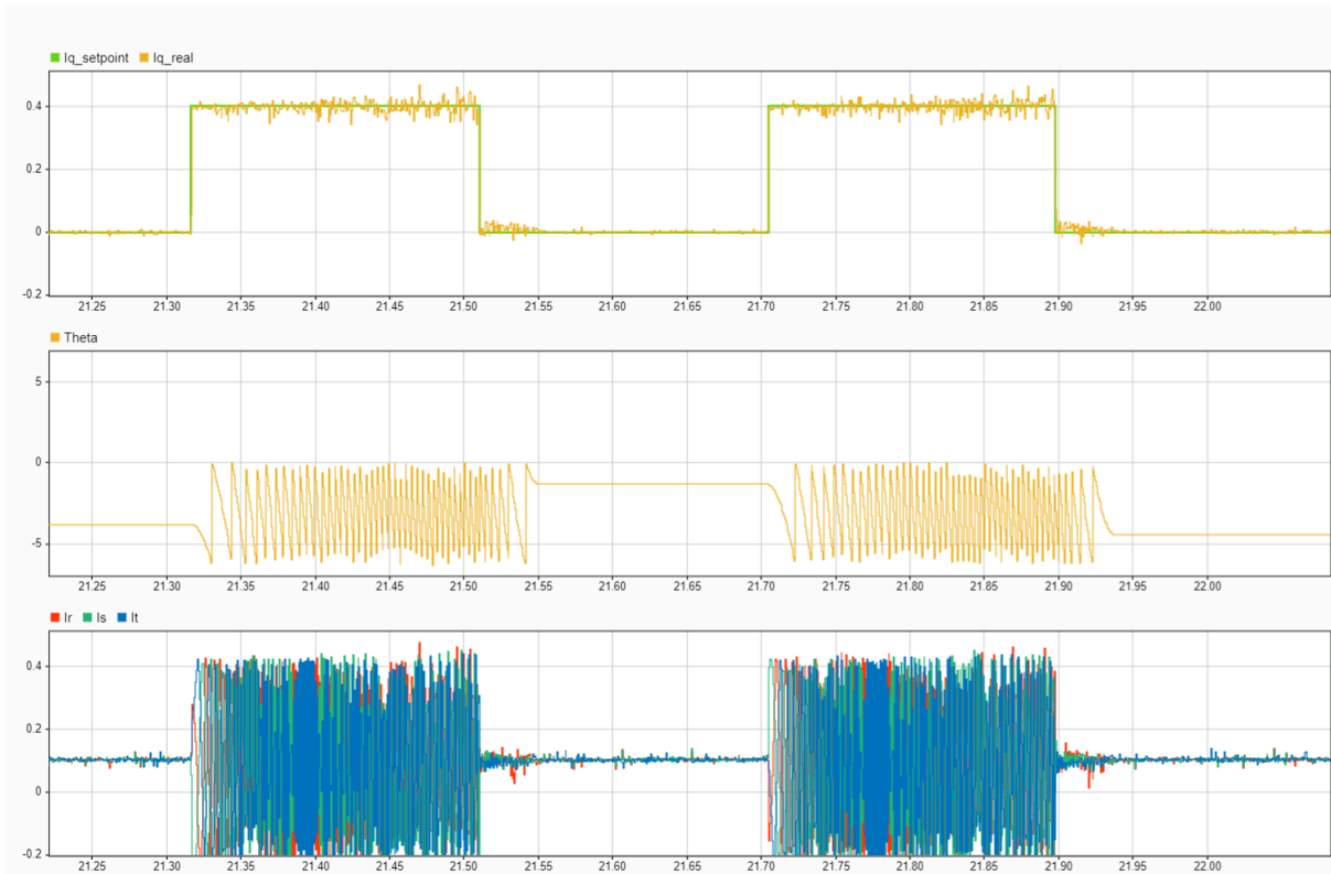
Fig. 48 - Experimental Test 3: Setpoint I_q vs. Real I_q [A], \Theta [rad], I_r, I_s, I_t [A]
