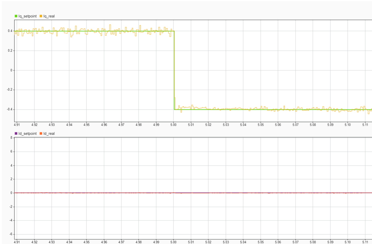
Fig. 46 - Experimental Test 2: Setpoint I_q vs. Real I_q [A], Setpoint I_d vs. Real I_d [A]
