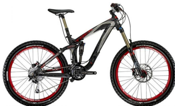
Figure 16. Example of mountain bicycle with double suspension. Source [19].
