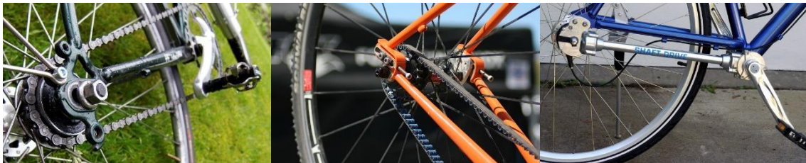
Figure 6. Transmission system examples. Left: Chain transmission; Center: Belt transmission; Right: Shaft transmission. Source: [2].
