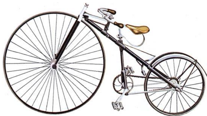
Figure 7. The "bicyclette" invented by Henry John Lawson in 1879. Source: [9]
