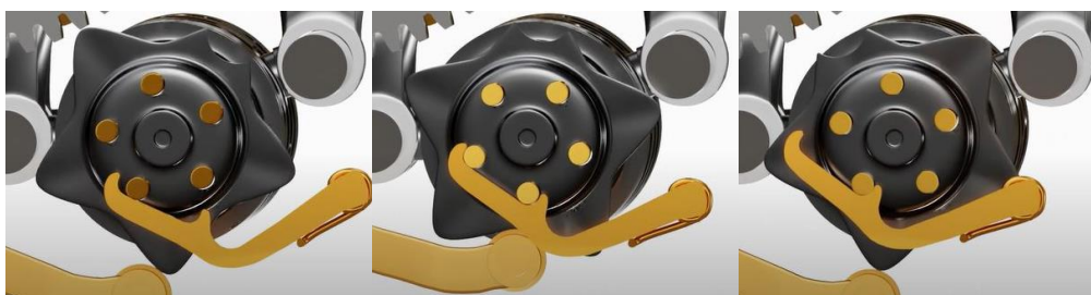
Figure 30. Explanatory pictures of the ratchet mechanism of a selector drum. Source: [41].
