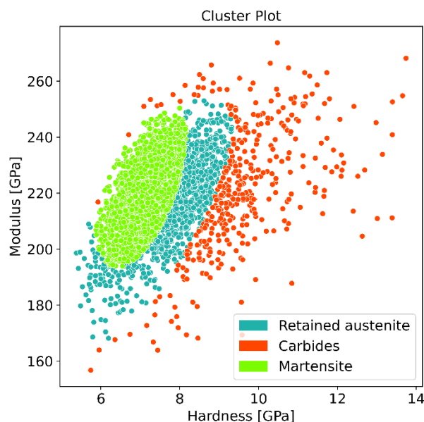
Figure 25: modulus in function of hardness representation of the phases identified by the clustering algorithm for the V4E region of the 316L+V4E transition sample. Source: author image.
