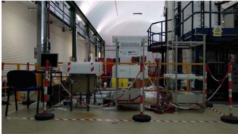
Figure 1. The High Efficiency Neutron Spectrometry Array HENSA at the LSC Hall A.
