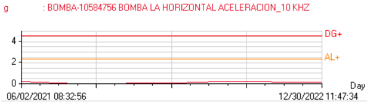
Figure IV.20. Pump bearing acceleration compared to the alarm and stop levels at G2I [38]
