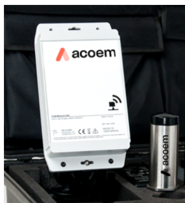
Figure 5.2.3. Acoem accelerometer and acquisition system [20]
