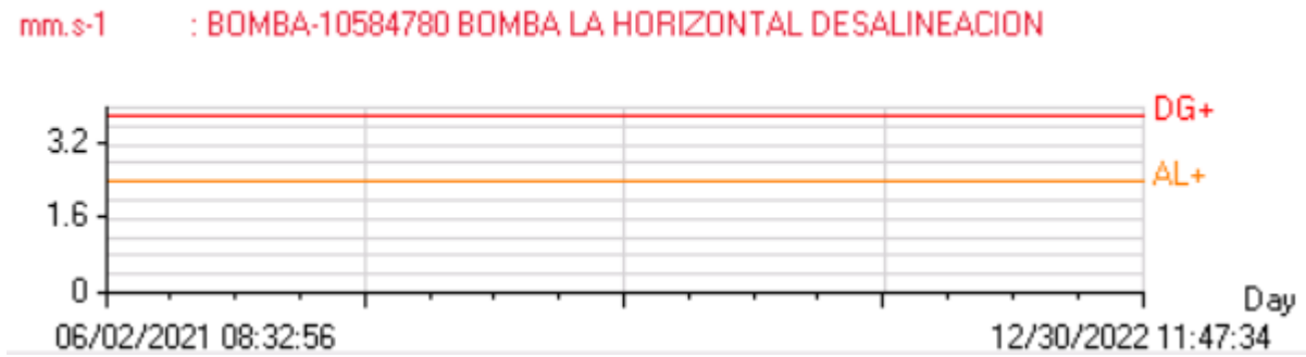
Figure IV.14. Pump bearing misalignment compared to the alarm and stop levels at G1II [38]
