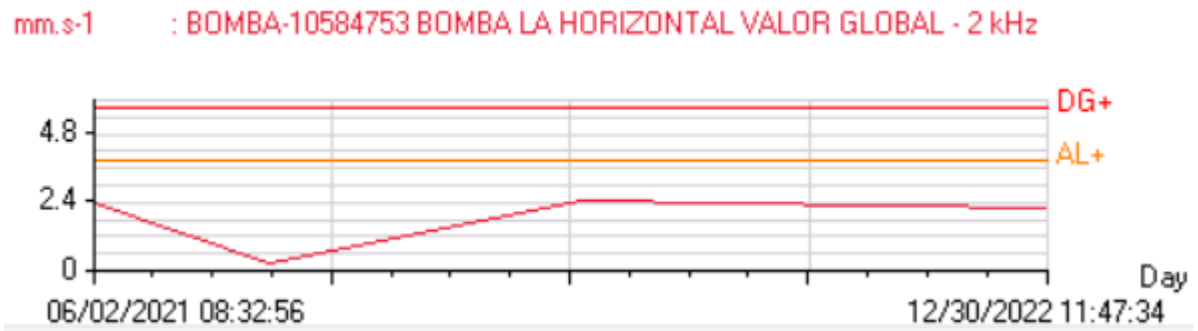
Figure IV.50. Pump bearing global status compared to the alarm and stop levels at G1I [38]
