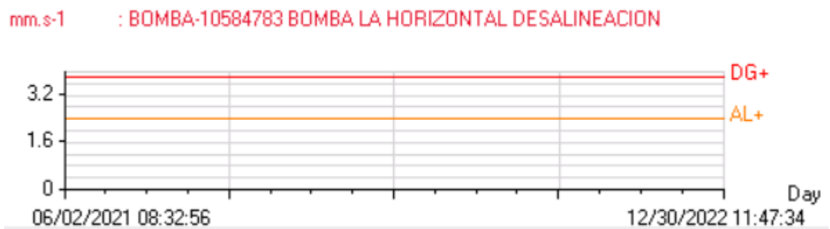
Figure IV.16. Pump bearing misalignment compared to the alarm and stop levels at G2II [38]
