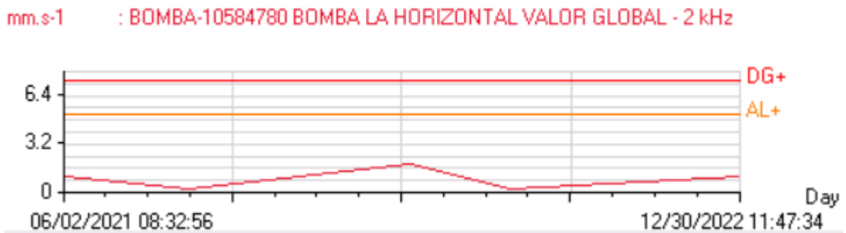
Figure IV.54. Pump bearing global status compared to the alarm and stop levels at G1II [38]
