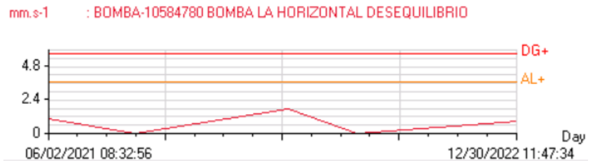
Figure IV.6. Pump bearing unbalance compared to the alarm and stop levels at G1II [38]
