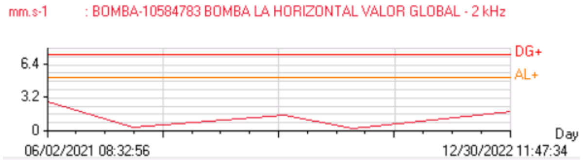
Figure IV.56. Pump bearing global status compared to the alarm and stop levels at G2II [38]
