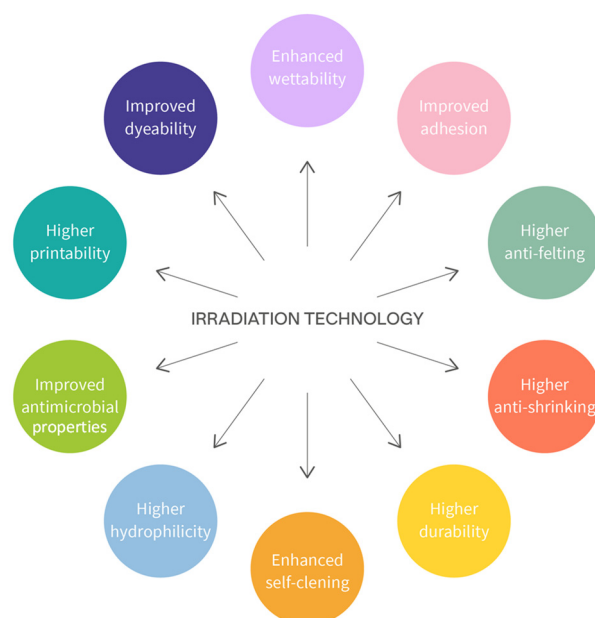
Figure 4. Possible effects of irradiation technologies on textile materials. Adapted from Islam and Mohammad [91].
