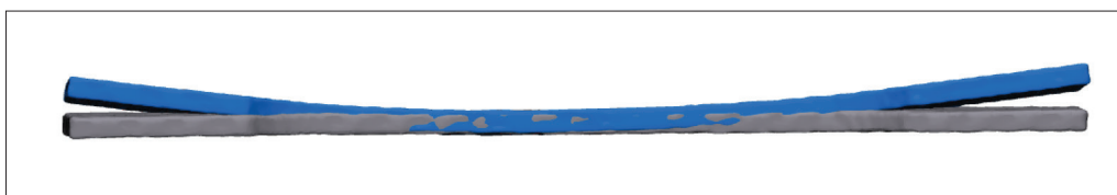
Figure 2. Prealignment between a MED610 control tensile (gray) and a MED610 tensile that was sterilized with AU134 method (blue).
