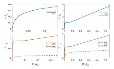
Figure 1. The relationship between the local multiplicity  $(E_2)_{uu}[(E_N)_{uu}]$  and  $\Delta\lambda_2$  [ $\Delta\lambda_N$ ] caused by the removal of node u, in networks with BA, WS and ER topologies. Results are averaged over 1000 iterations.
