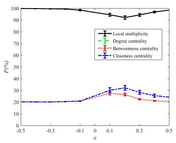
Figure 5. Precision in finding the node whose removal causes a maximum impact on algebraic connectivity in random ER networks with wiring probability p=0.5 and different assortativity level  $\sigma$ .
