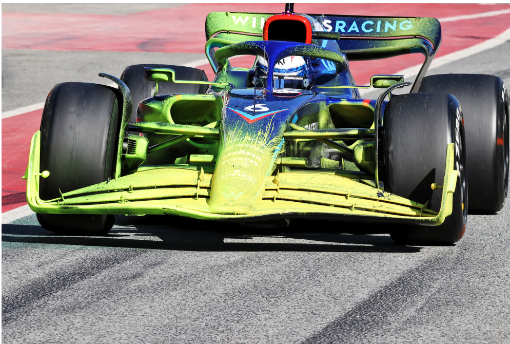
Figure 2.4: Nicholas Latifi's Williams FW44 covered in Flow-Viz during pre-testing of 2022 season in Barcelona. Source: SkySports.
