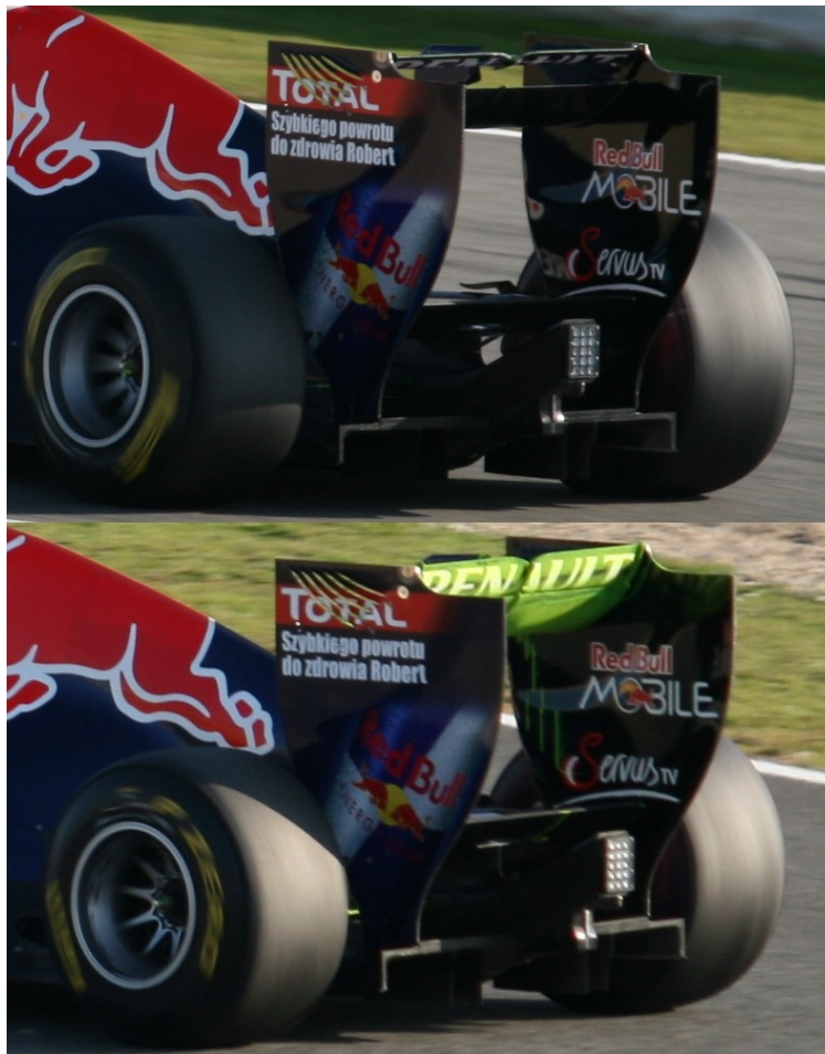
Figure 2.11: Redbull's RB7 DRS system. Source: Gil Abrantes.
