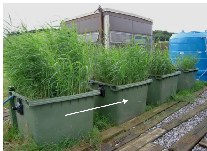
33 34 35 Fig. 1 Pilot-scale tidal flow constructed wetlands system
