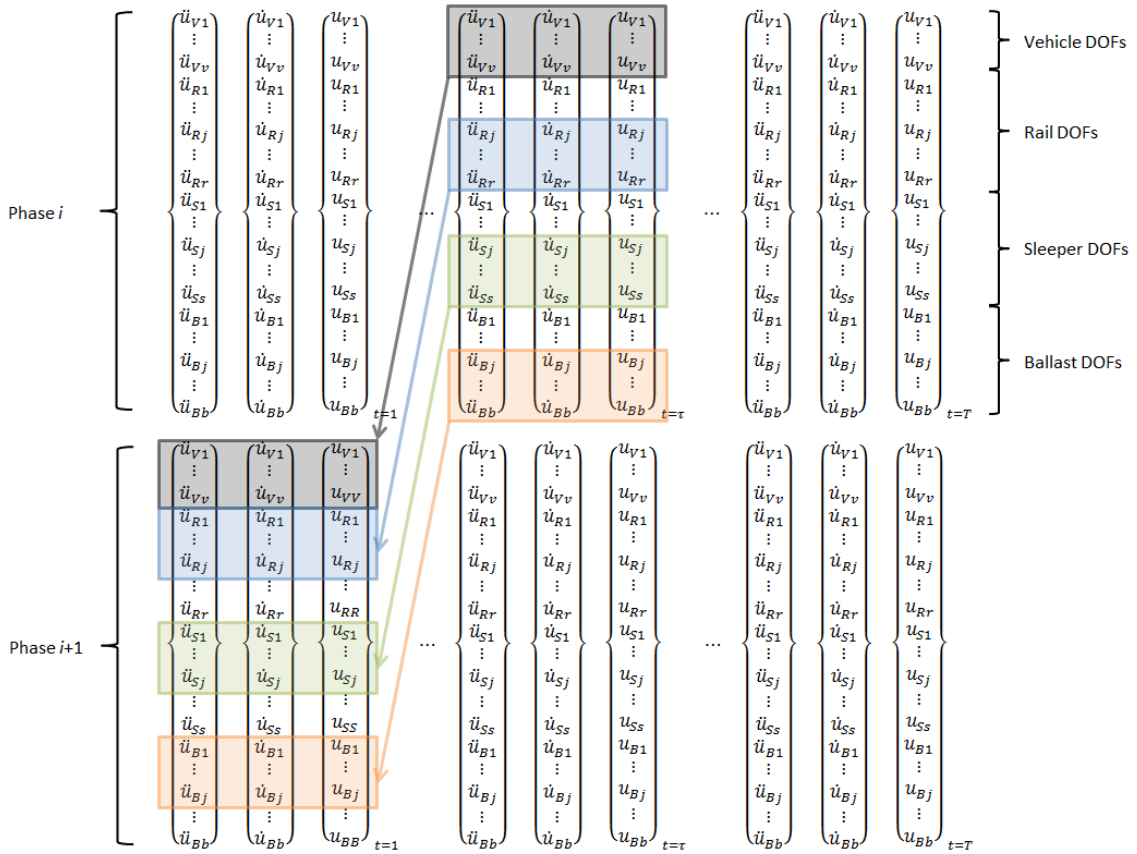
Figure 9. Transfer of state vectors for Model B. Shaded areas: Vehicle DOFs – subscript V; Rail DOFs – subscript R; sleeper DOFs – subscript S, ballast DOFs – subscript B
