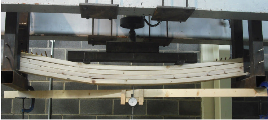
Fig. 10: Four – layer 44-dowel beam at failure
