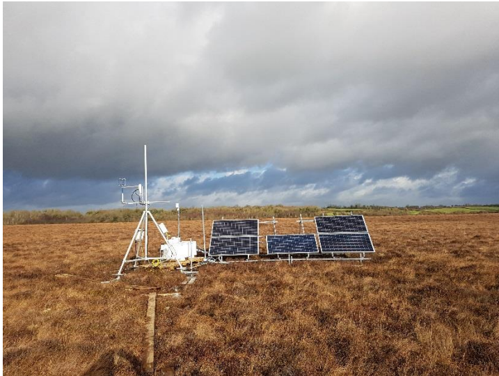
Figure 4.17 Example of an eddy covariance tower at Clara bog, Co. Offaly, Ireland.
