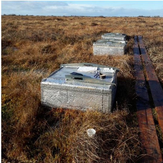
Figure 4.3. Dark chambers used for measuring methane (CH 4 ) and nitrous oxide (N 2 O) fluxes.
