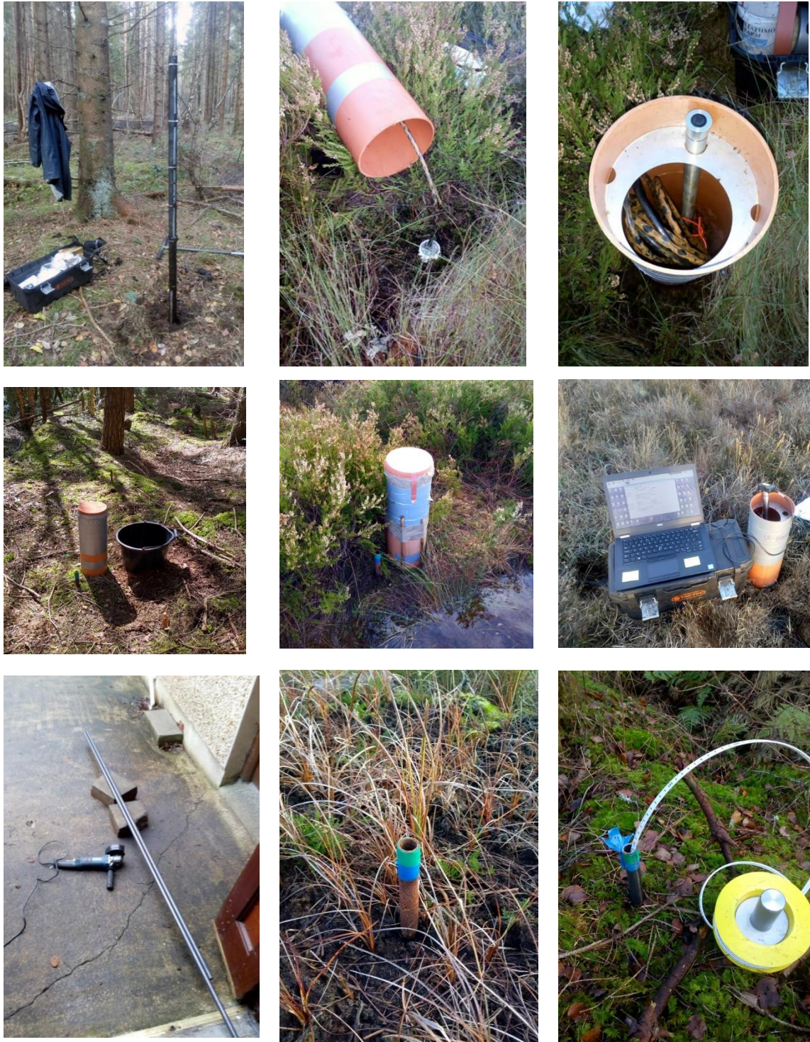
Figure 3.2.5. Equipment used for high-frequency hydrological monitoring: Top row – preparation and installation of high-frequency water level loggers at a sampling location. PVC-tubes were installed in augered holes (left), loggers were inserted into tubes (centre). Orange PVC tubes (diameter 150 mm) were used as mounts for the communicator devices of the loggers (right). Middle – Monitoring stations at drained (left) and rewetted (centre) raised bog in Scohaboy. Monthly calibration of loggers, and data download of logging data (right). Bottom – Manual hydrological measurements: Preparation of iron rods (left), installed rod at a domestic extraction site (centre), and measurement of water table depth using water level probe (right).
