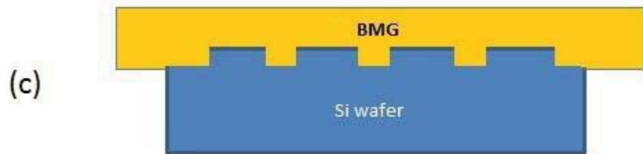
Fig.1 (a) Photoresist laid down on silicon wafer, (b) Deep reaction ion etch and remove photoresist, (c) emboss silicon into BMG above glass transition temperature of BMG, (d) remove silicon by dissolution, (e) use BMG as tool to emboss a polymer at temperature below glass transition temperature of BMG, (f) withdraw BMG tool from polymer. Using this route allows a single silicon master to produce one BMG tool which can then produce Y number of plastic components.
