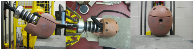
Figure 1. Hybrid III reconstruction of a fall.
