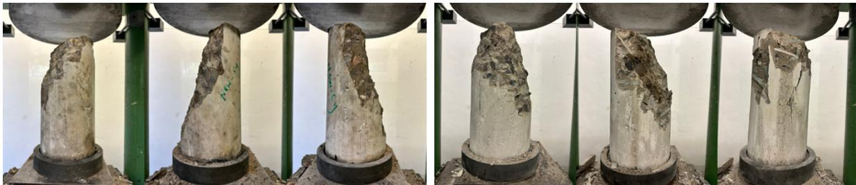
a) Failure pattern for control samples.
