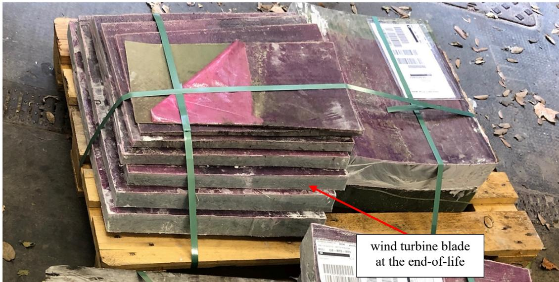
Figure 1: FRP wind turbine blade section before processing to FRP needles.
