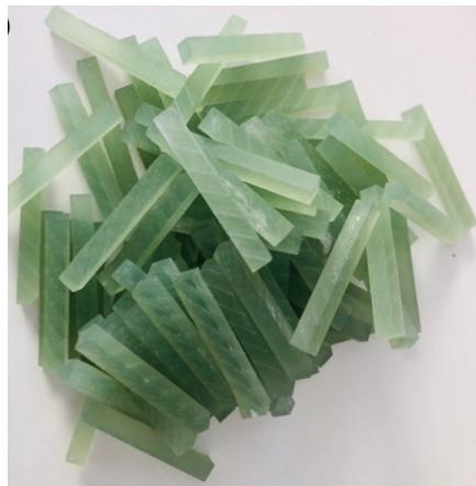
Figure 2: FRP needles produced.
