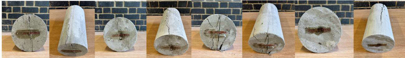
b) Fracture patterns of FRP-RA-2.5 samples.
