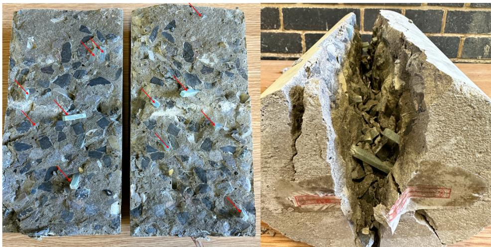
Figure 10: Fractured surface of an FRP-RA-2.5 specimen.
