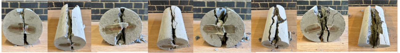
a) Fracture patterns of control samples.
