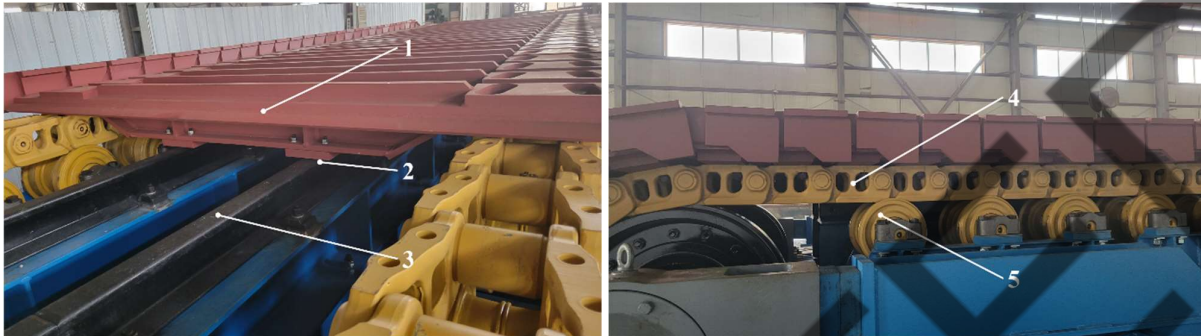
1.Bearing plate; 2.Plates and rail contact position; 3.Support guide rail; 4.Traction chain; 5.Support wheel
